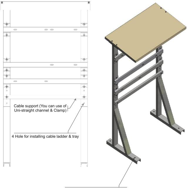
Installing on ground with roll-bolt M20
